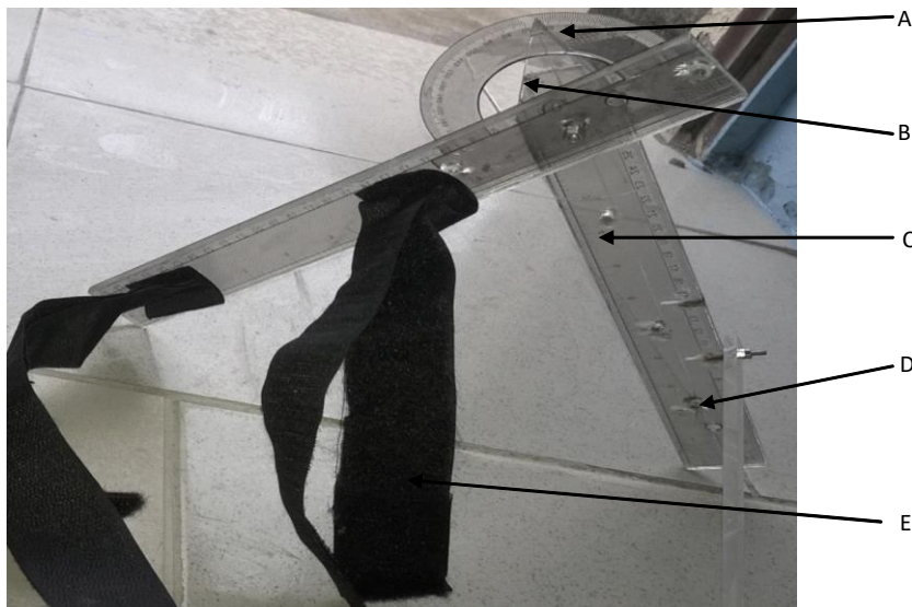
Figure 2: Photograph of the Newly Developed Device (A = the protractor graduated in degrees (the arm); A= the immovable arm (disc); E = the Velcro straps, D = the perpendicular arm (stud) and B = the movable arm).
