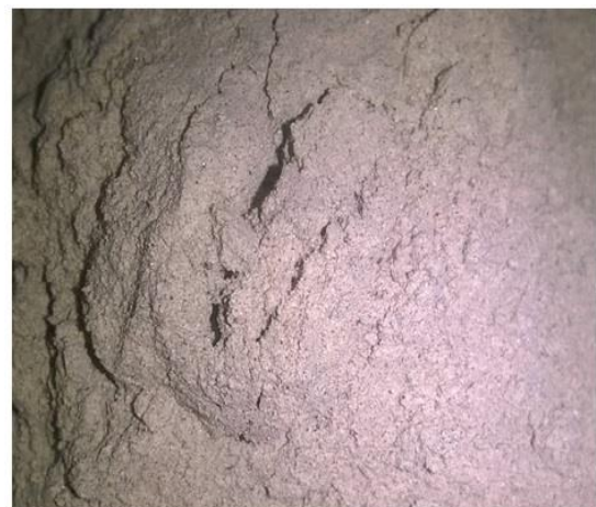
Fig. 1. Picture of 80 µm quarry tailings particles
