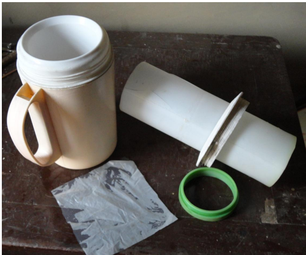
Figure 3. Components of the aerofloral sampler – flask base, plastic cylinder, 5 \mu sieve and sieve clamp.
