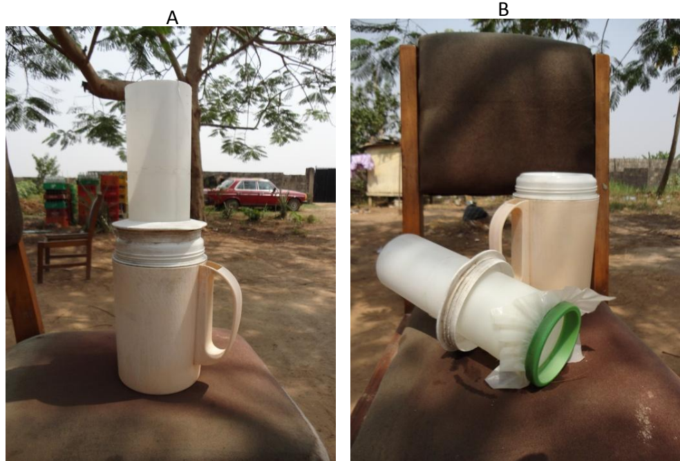
Figure 2. Aerofloral sampler on display (a), and dismantled (b) showing the sieve-clamped cylinder and the basal flask.
